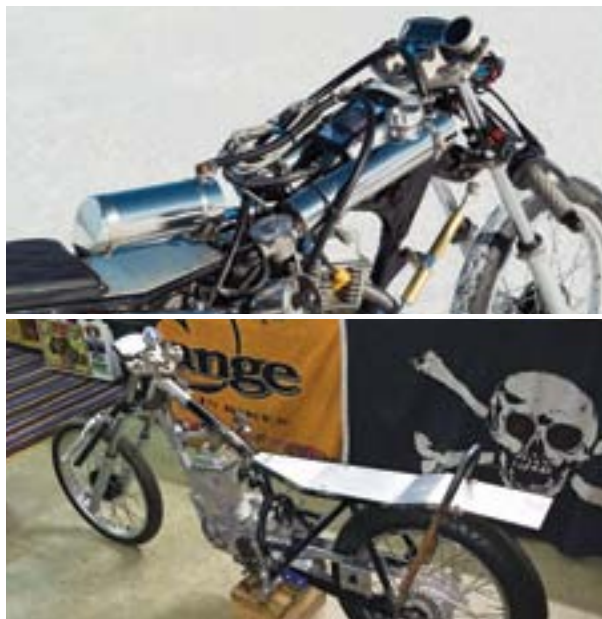
Left: The bike had its shock removed in favour of a fully rigid subframe. The tanks in front of the seat hold a mixture of high-octane gasoline and ethanol. And yes, there's a steering dampener!
