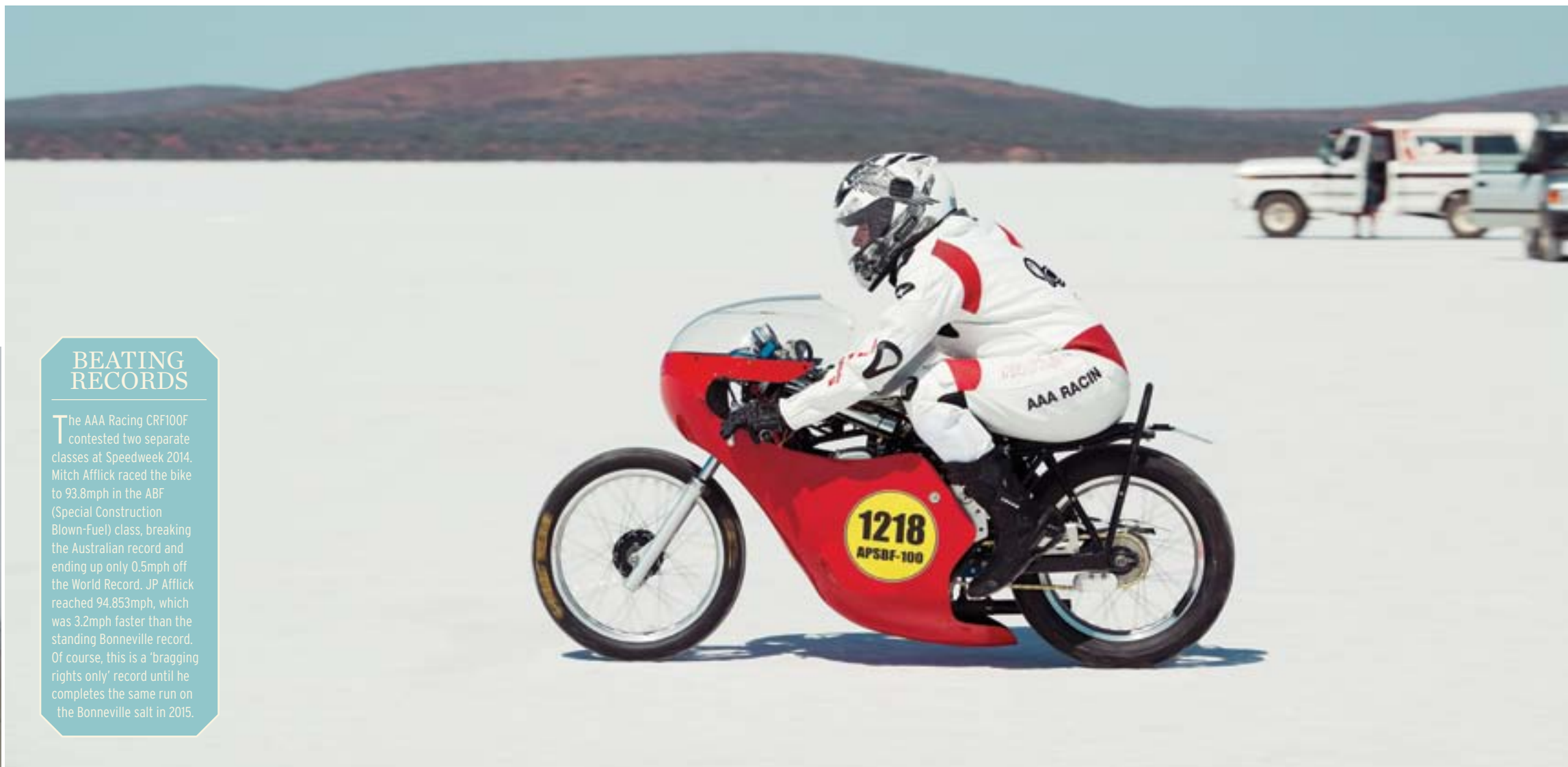
Left: The bike had its shock removed in favour of a fully rigid subframe. The tanks in front of the seat hold a mixture of high-octane gasoline and ethanol. And yes, there's a steering dampener!
